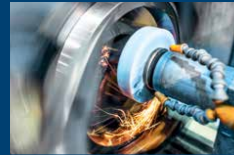
7. Inner Diameter Circular Grinding
